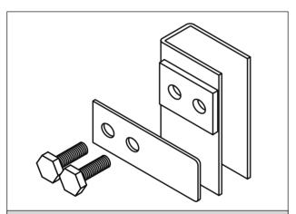
**15** Attach the stops to the guide channels (as shown above) and if applicable attach handles to the bottom slat.
