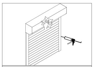
**17** To complete the installation you should mastic around the edges of the shutter then give the shutter a final clean and tidy.
