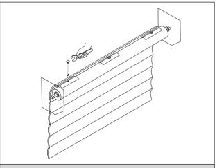
**11** Attach the curtain to the axle using the attachment strips provided.
