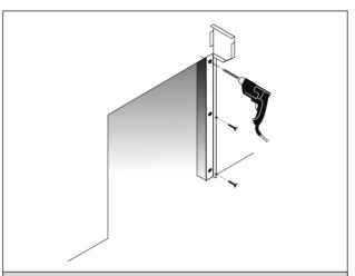
**3** offer angle up and fix to wall ensuring vertical (use all fixing holes provided)
