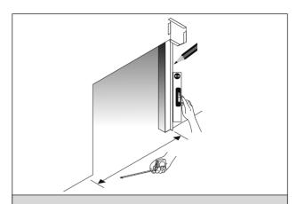
**2** Measure the opening to determine the location of the first length of angle. If the floor is sloping you must fit the higher side first. Fix the angle to the wall.
