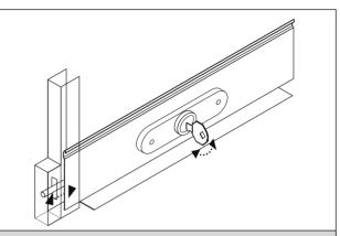
**8.** If a lock has been supplied in the bottom slat you should remove the bottom slat from the curtain. Slide the bottom slat down into the guide rails and check that the lock bars in the bottom slat will locate into the prepared guide rail keeps. Enlarge the keeps if necessary.
