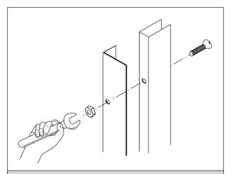
**1** The channels are supplied with the angles attached these must be removed.
