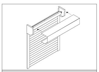
**16** If required fit the hood / fascia. If the shutter is externally fitted the hood / fascia should be fastened using appropriately coloured 4mm rivets.
