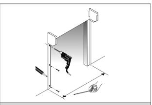
**4** Measure from the first angle to determine the position of the second angle ensuring that the angles are vertical and also that the tops of the end plates are level. Fix the angle to the wall.
